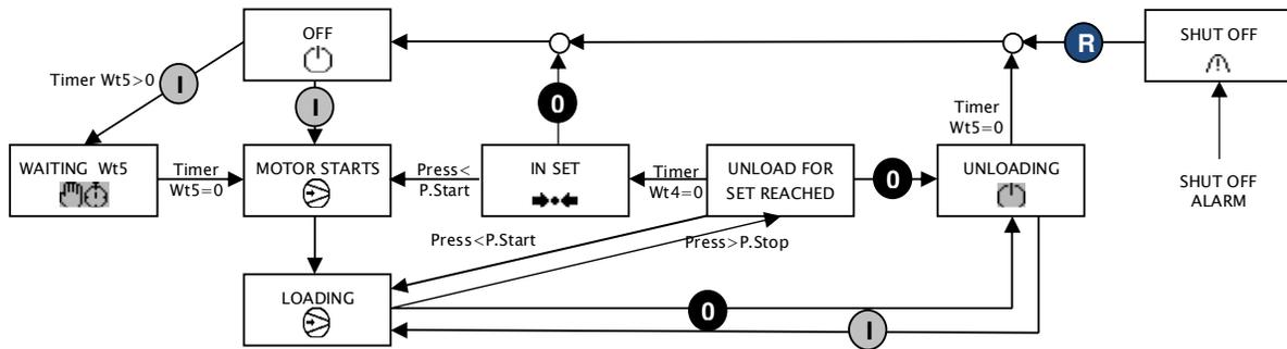
The symbols into the above squares indicate the compressor status showed on the main visualization of the LCD. The back is grey while the symbol is blinking.
