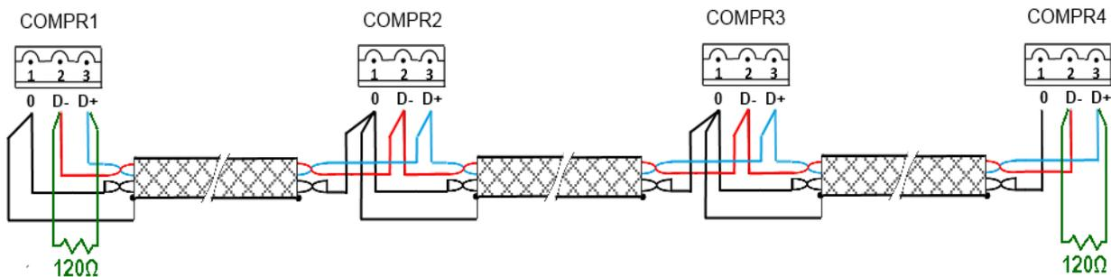
**NOTES ON THE WIRING: wrong wiring can damage both the controller and other devices connected to the serial port.**
